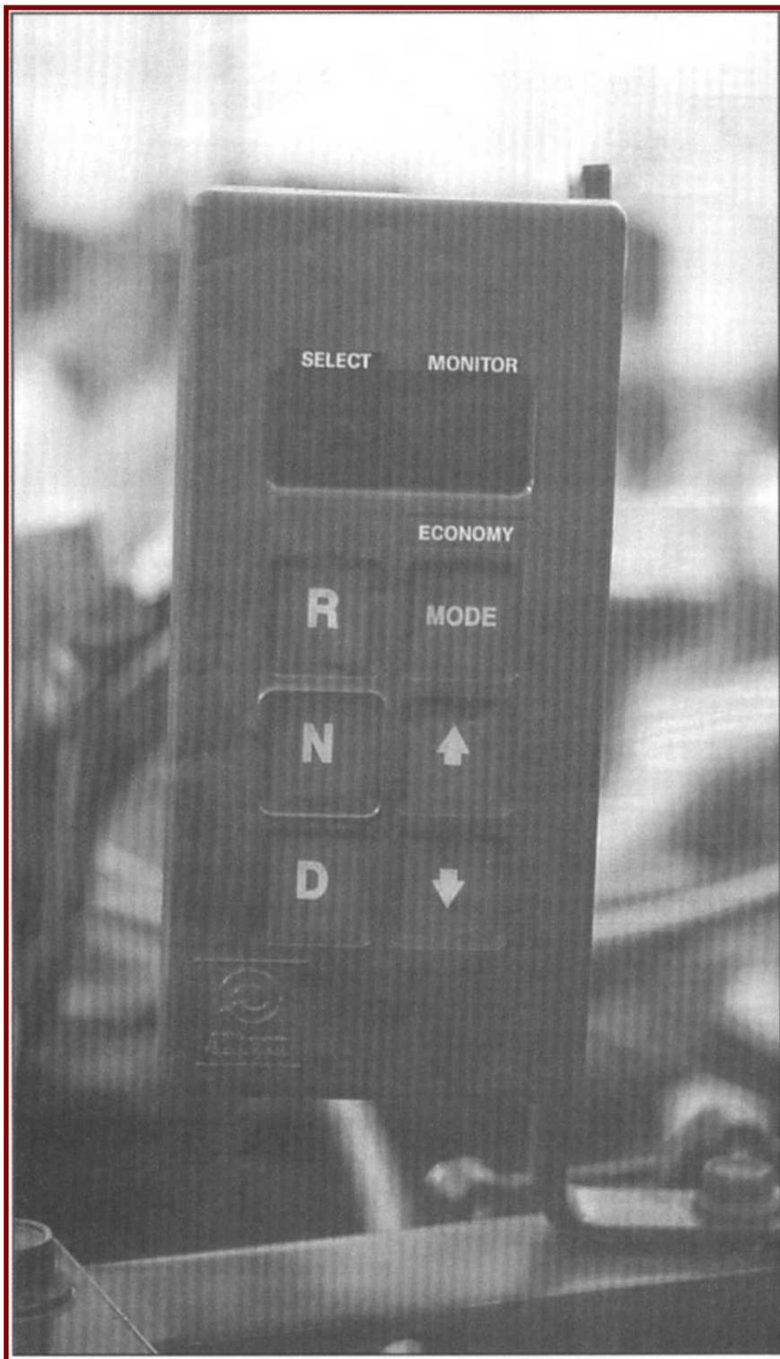
The touch pad commonly found in motorhomes equipped with this transmission is more than just a gear selector. It serves as a communication link between the transmission and the operator.
