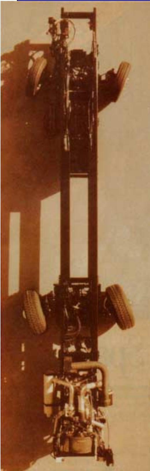
*With the All-Steer chassis in the "coordinated steer" mode, the front and rear wheels of the vehicle can turn in opposite directions which is said to decrease the turning radius of the chassis by nearly one-third*
