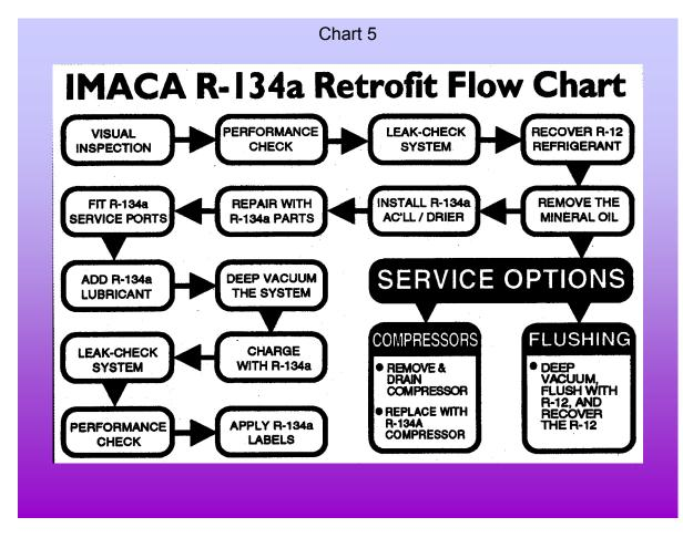
sion to an alternative refrigerant should be considered. Many repair facilities, may service only a limited number of refrigerants, so the choice should be given careful consideration.
