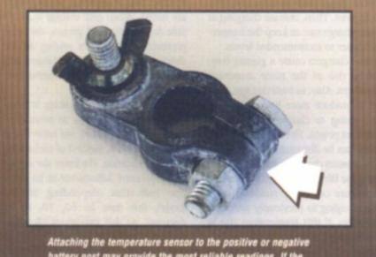
Attaching the temperature sensor to the positive or negative battery post may provide the most reliable readings. If the battery has a lead post, the temperature probe can be inserted between the open ends of the battery cable where it is bolted to the positive post (arrow indicates insertion point).
